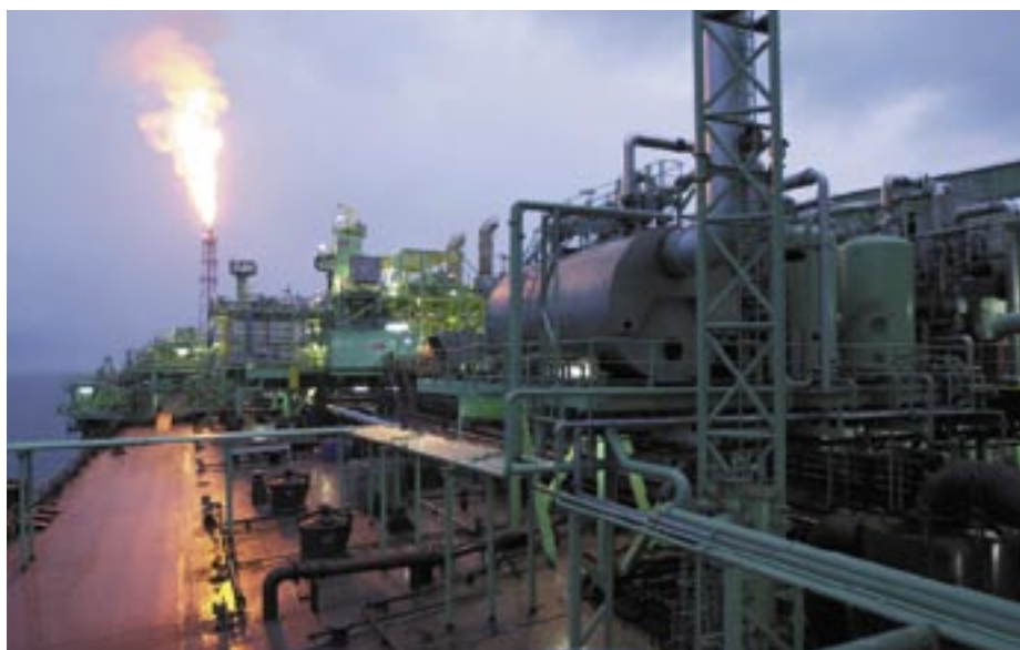
Giant floating production and storage vessels (FPSOs) makes expensive on-shore production and storage infrastructure unnecessary.
